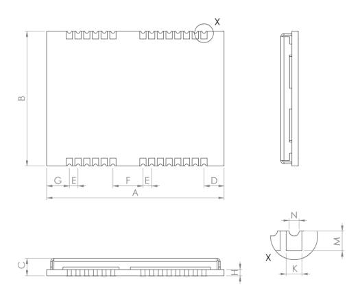
Figure 3-1 Mechanical Layout
