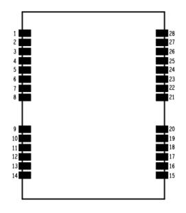
Figure 3- 2 UM220-IV L Pin Assignment
