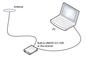
Figure 2- 1 Typical Installation of UM220-IV L
