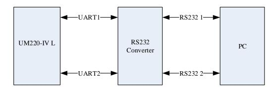
Figure 4-8 Connect to PC through UART
