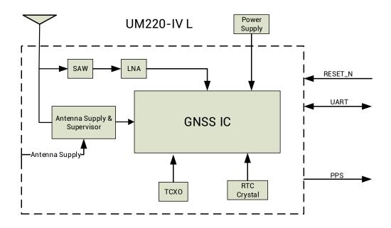
Figure 1-1 UM220-IV L Block Diagram
