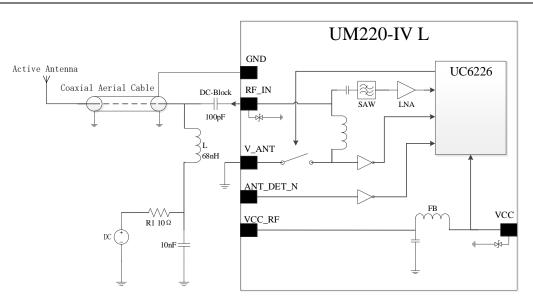
Figure 4- 4 UM220-IV L Active Antenna Solution Powered by External Power Supply
