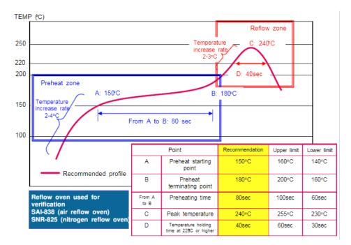
Figure 6-1 Reflow Soldering Curve
