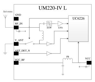
Figure 4-1 UM220-IV L Passive Antenna Solution
