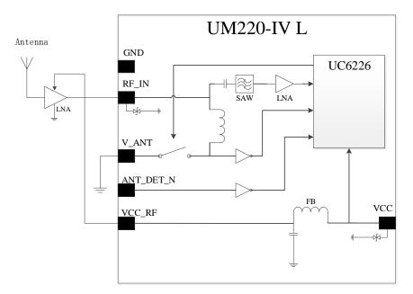
Figure 4- 2 UM220-IV L Passive Antenna High-performance Solution
